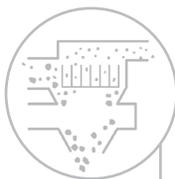
All Prater Air Classifiers separate particles based on the opposing principles of centrifugal force and aerodynamic drag force. As product enters the primary air inlet, individual particles are subjected to aerodynamic drag forces by the conveying air. This drag force varies with the size and density of the individual particles.
